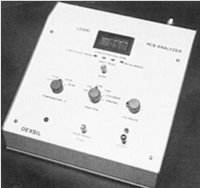
The PCB Analyzer can be used on transformer oil, soil samples, and for testing of total chlorine levels in waste oils.
